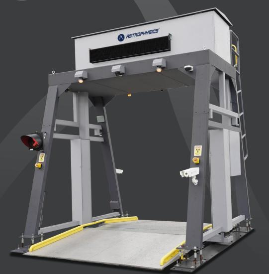
The HXC-LaneScan<sup>TM</sup> is a drive-through x-ray system designed to help detect weapons, explosives, and other contraband in motor vehicles. With a 320kV generator capable of penetrating 75 mm (3") of steel, it allows operators to identify threats in nearly every space of a vehicle, including the wheels, glove box, trunk, and spare tires.
